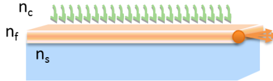
Figure 1.2.- Waveguide along which light propagates. n_c : cover layer refractive index; n_f : film refractive index; n_s : substrate refractive index ( n_c < n_f < n_s ).
